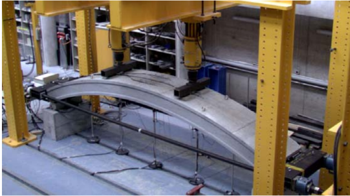
Figure 12: Full scale load tests on precast tunnel segment
