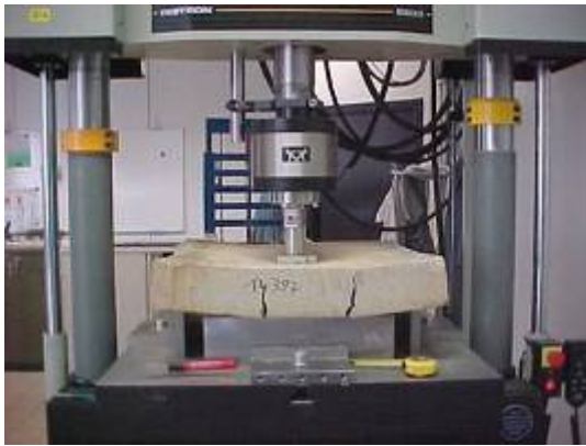
Figure 8: Testing of an EFNARC Panel
