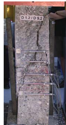
Figure 14: Tests set-up on joint connections between segments
